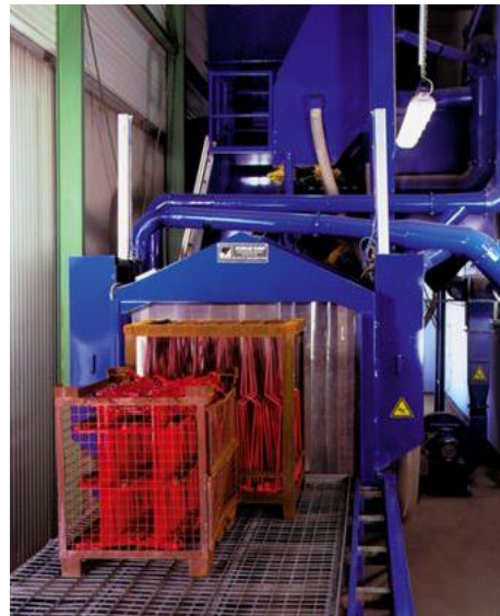
Continuous-feed blasting unit, 35 m long
