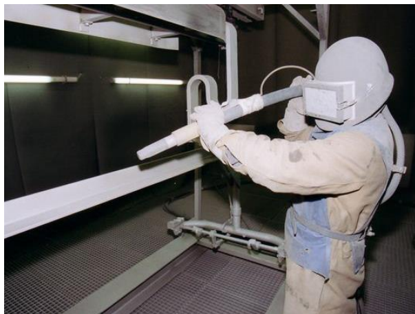
Blasting station (shot-blasting technology)
