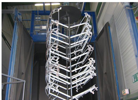
Shot-blasting equipment with overhead conveyor
