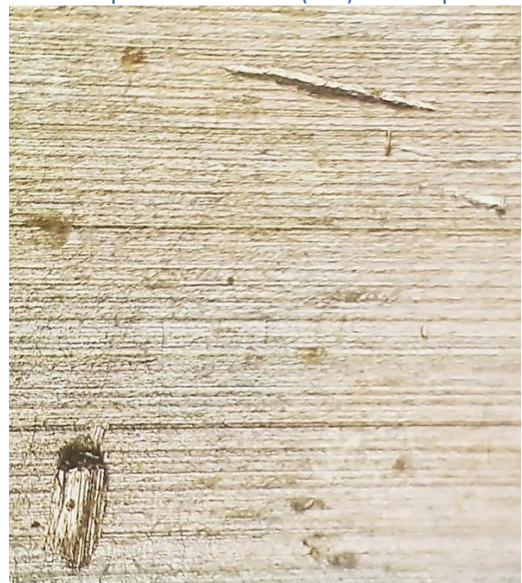
Metallic particles inclusion (40X). Unacceptable
