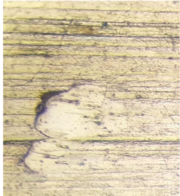
Metallic particles inclusion (40X). Unacceptable
