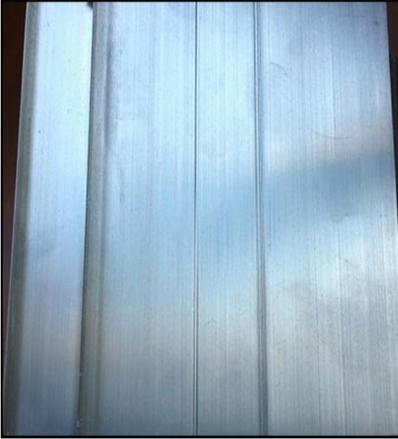
Streaks and tearing(40X). Unacceptable
