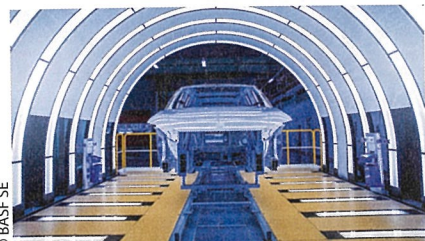
Aluminum body with thin-film pretreatment, cathodic dip coating, water-based filler, water-based paint, and a two-component clear coat.
