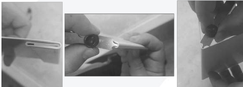
Figure 10 - Bend test for postforming - pressing and measurement
